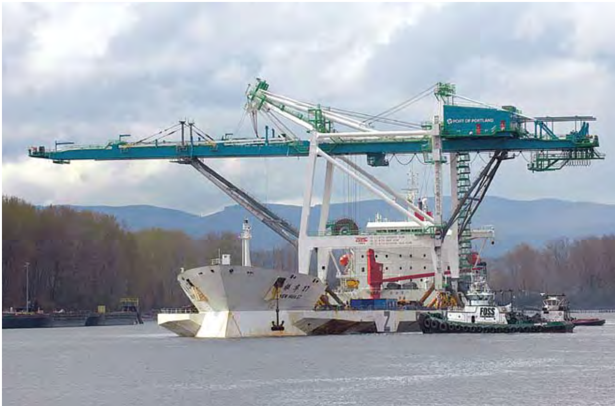
The new post-Panamax container crane makes its final approach to Terminal 6 following a month-long journey from China.
