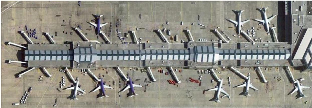
**Building Description:** Concourse C is a two-story structure with roof mechanical penthouses. It is divided into three separate structures, each with similar construction, but separated by seismic joints. Concourse C was constructed as part of the Terminal Expansion South projects in the late 1990's.
