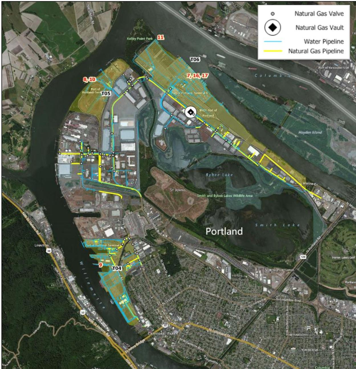
**Figure 17: Onsite Natural Gas and Water Pipelines at Terminals 4, 5, and 6 (Sources: Port of Portland)**
