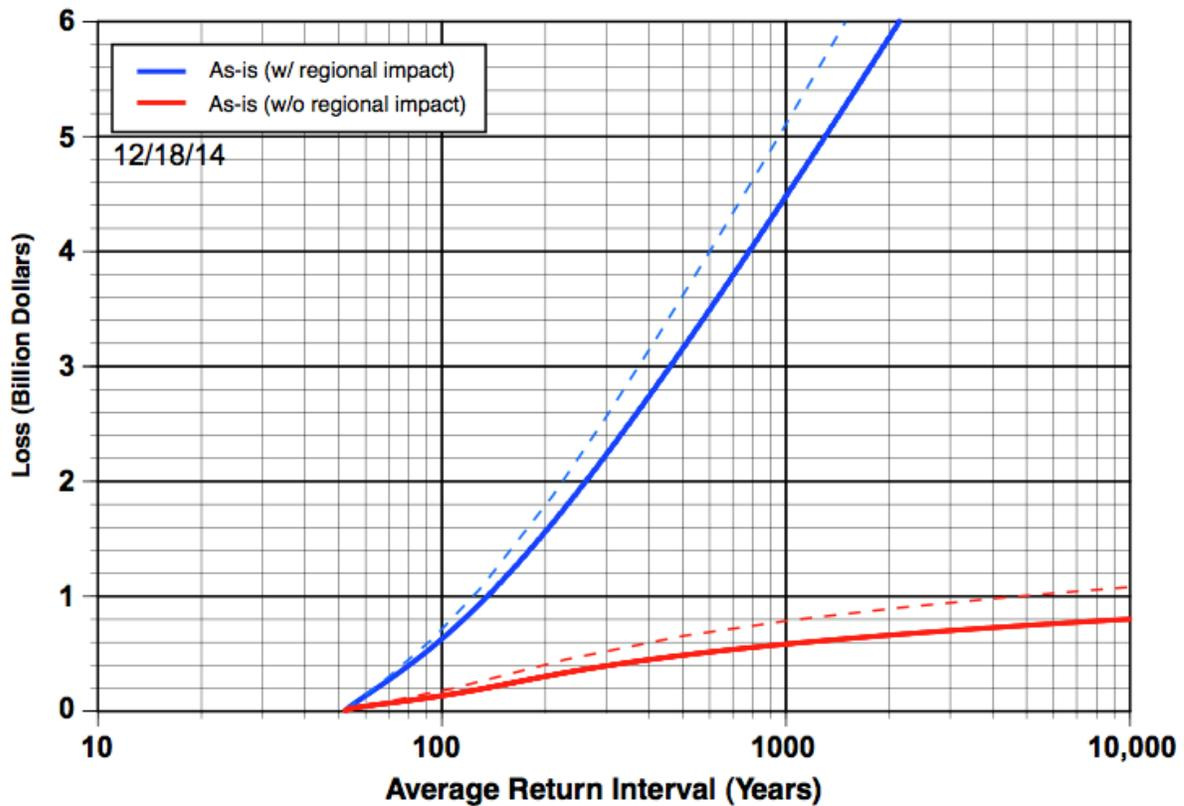
Figure 4 – Seismic Risks to Critical Facilities, As-Is
