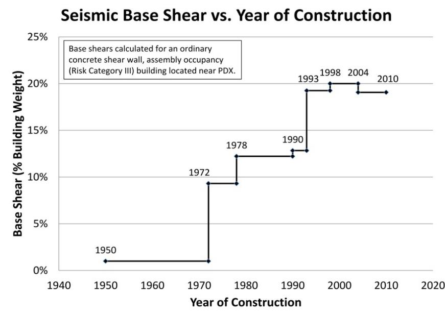
**Figure A – Increase in Building Code Seismic Loading Requirements as applied in Oregon (prepared by KPFF)**
