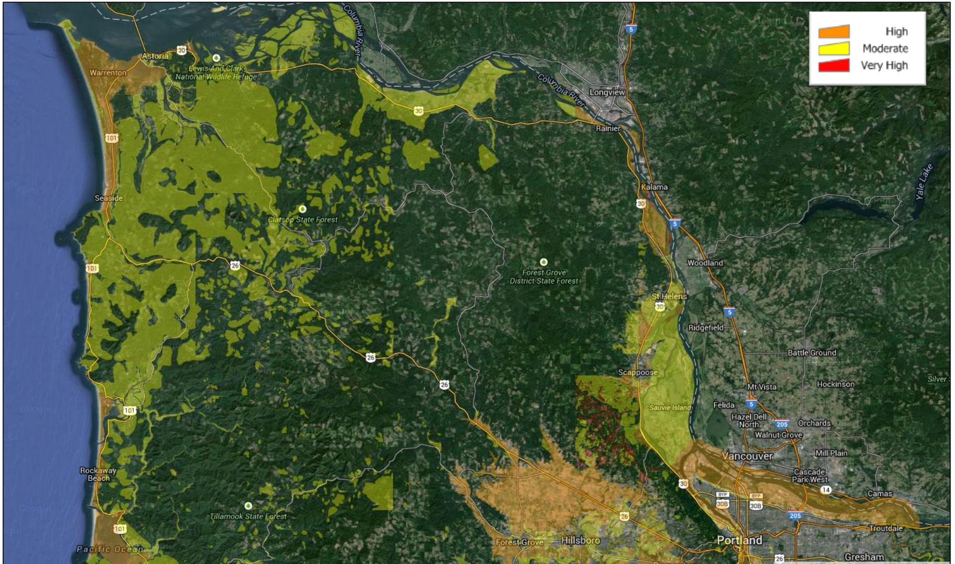
**Figure 12: Liquefaction Susceptibility throughout Oregon (Source: Oregon Department of Geology and Mineral Industries, DOGAMI. Note, data does not include the State of Washington)**
