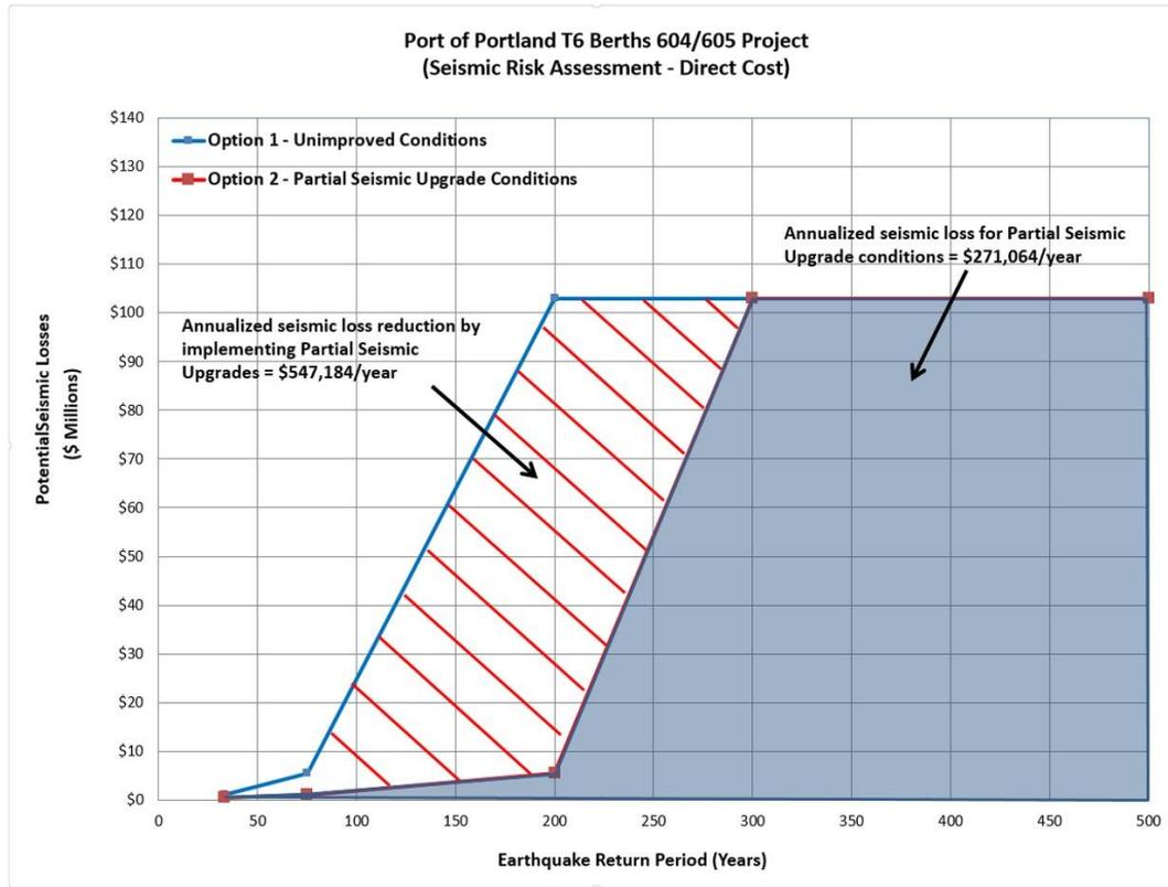
**Figure 12 – Berth 604/605 partial seismic retrofit annualized seismic loss reduction**
