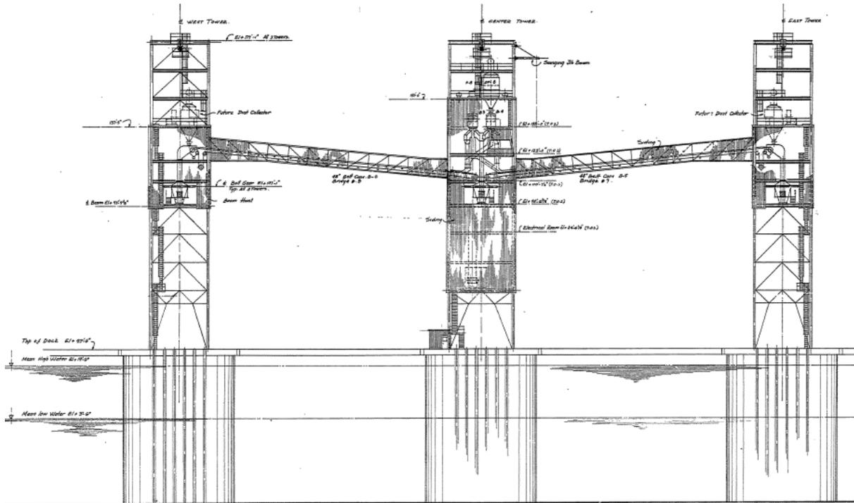
**Figure 5 – Berth 501 cell structures and shiploader towers elevation**
