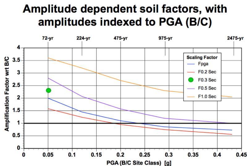
**Figure 6 – Site-Specific Ground Motion Scaling Model for PDX**
