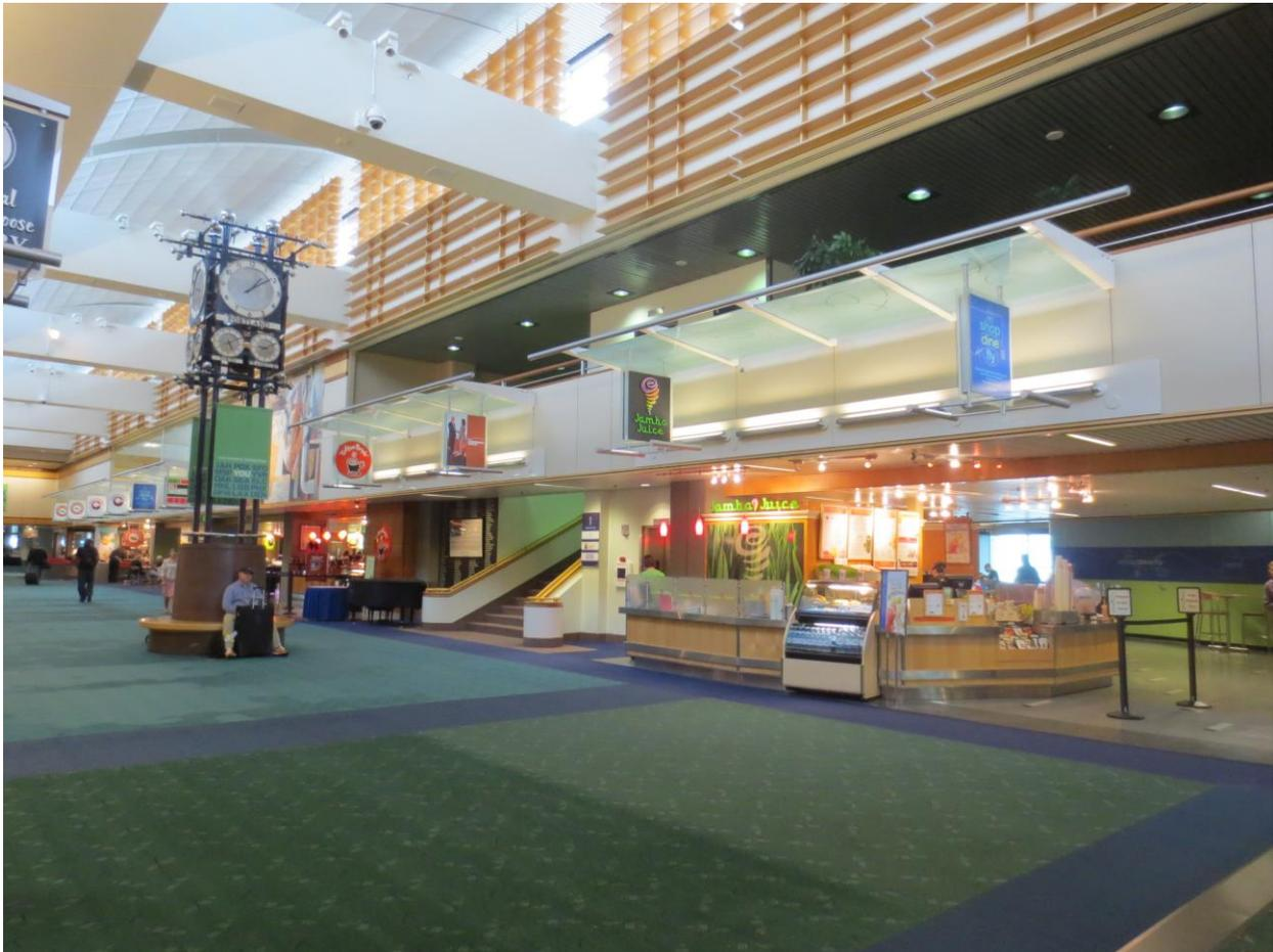
**Building Description:** The central portion of the Oregon Market Place is a three-story structure including the mezzanine. It consists of portions built in different construction projects, including the Oregon Market Place project that demolished a portion of the roof structure to add a raised clerestory.
