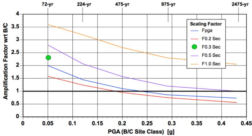
**Figure 2 – Site-specific ground motion scaling model for the Port**
