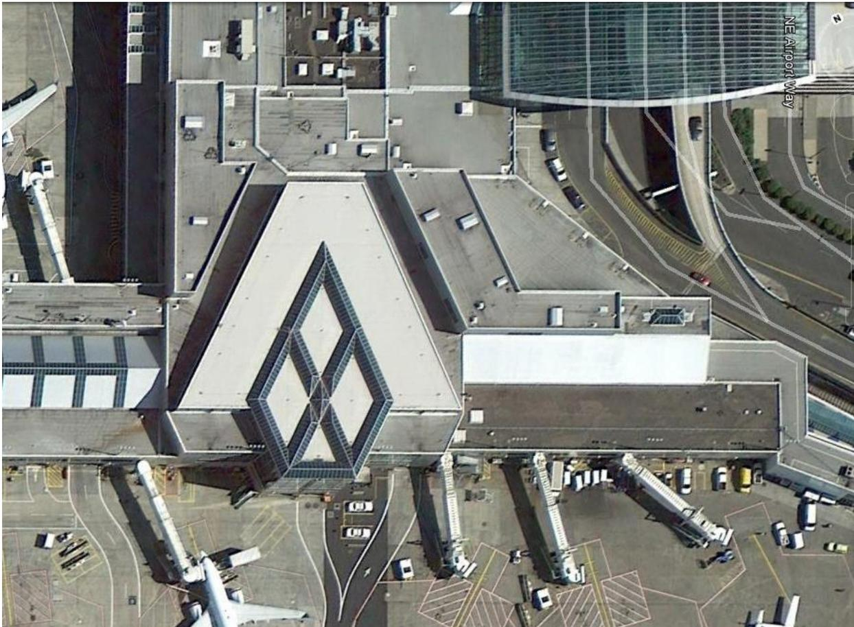
**Building Description:** The south node of the terminal is a three-story structure with mechanical penthouses on the roof. The central area is a two-story space with a steel space-frame roof structure.
