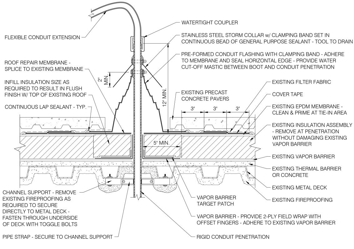
**EPDM FLASHING - ELECTRICAL CONDUIT** SCALE: 3" = 1'-0"
