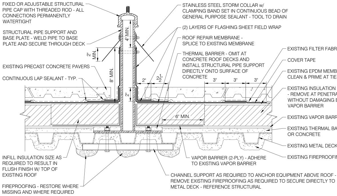
EPDM FLASHING - STRUCTURAL PIPE SUPPORT (FIELD WRAP) SCALE: 3" = 1'-0"
