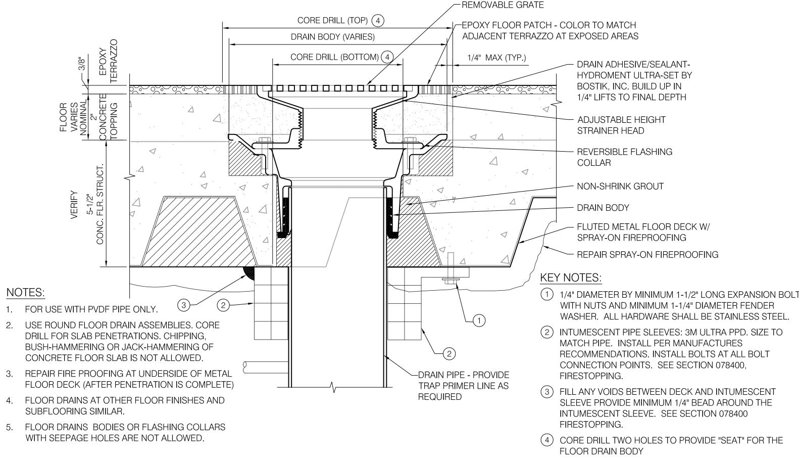
FLOOR DRAIN - COMPOSITE FLOOR - PVDF PIPE SCALE: NTS
