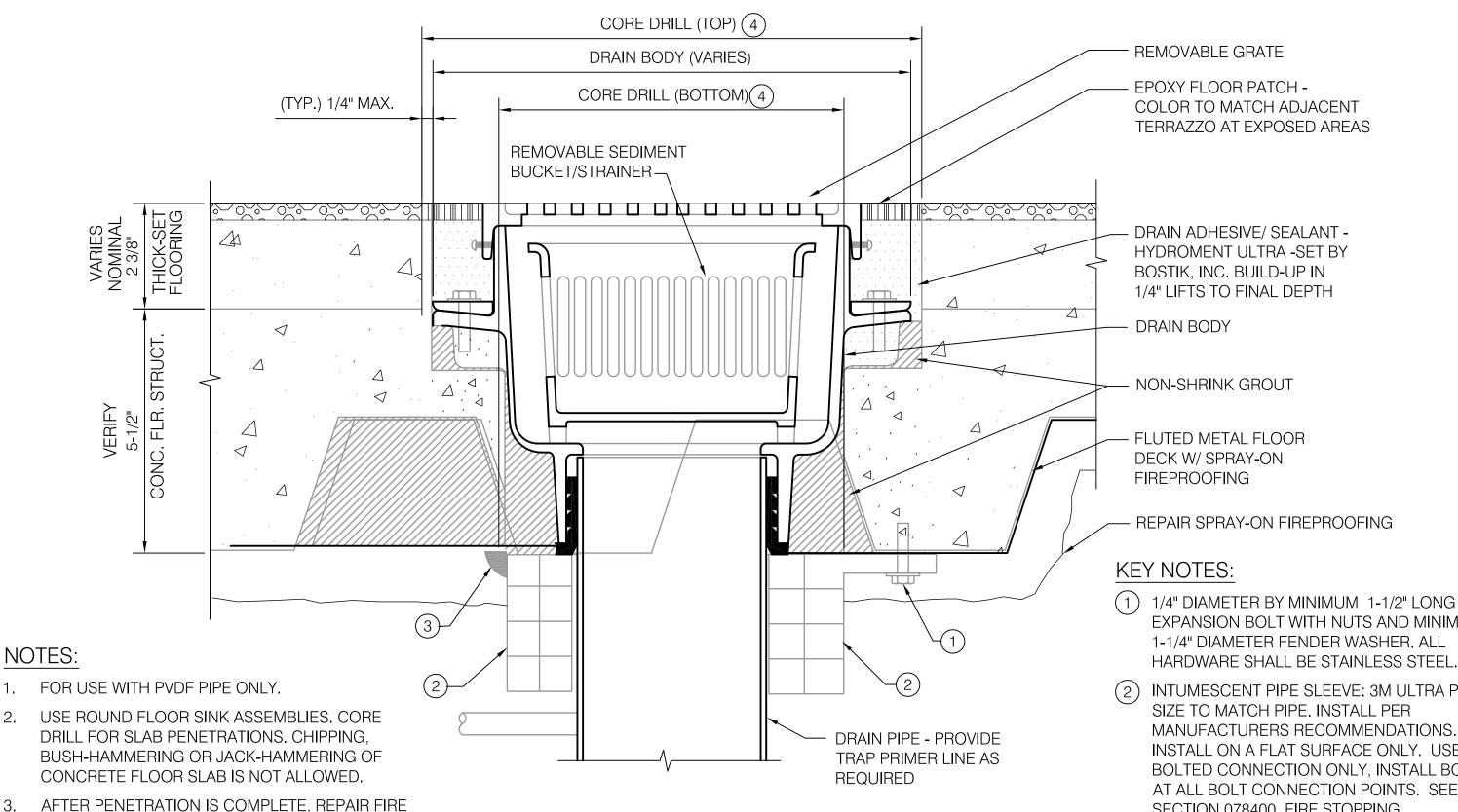
EXPANSION BOLT WITH NUTS AND MINIMUM 1-1/4" DIAMETER FENDER WASHER, ALL HARDWARE SHALL BE STAINLESS STEEL.
