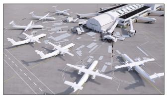
The good news is that project planners and engineers are making the temporary transition to C as smooth as possible. As you'll see in this rendering, the C-West jetways will rotate and include ramps for boarding from ground level. Deplaning passengers can take cover from rainy weather under a large tent and use a ramp or stairs to enter the terminal. For travelers with limited mobility, an elevator will be available.
