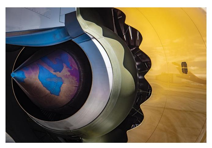
**From Brian**: Taken in May 2020, this is the back of one of the engines on a Gulf Air Boeing 787 that was painted at the PDX Boeing paint facility. The airplane has been sitting at PDX for months, a victim of the global aviation slowdown during COVID. The blue discoloration on the conical part of the engine is part of a natural metal oxidation process. Eventually, it will fade away.
